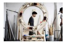
'The Thread Wrapping Machine is a tool to join different types of material with only a glue-coated thread to bond it. By using this construction method materials such as wood, steel, plastic or bricks can be joined to form objects and spaces.
