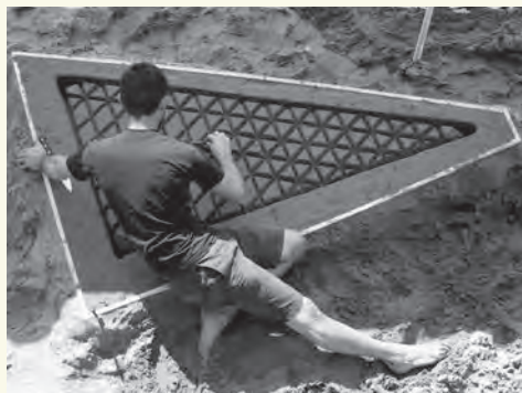
Pewter Desk (2011), a private commission for Calder Foundation president Sandy Rower, was hand-cast by Lamb and a group of students during low tide on Caerhays Beach in Cornwall, near where the designer grew up.
