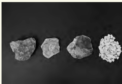
Material samples of the four Italian marbles used as the aggregate for Marmoreal each have a distinct color (from left to right): Rosso Verona (red), Giallo Mori (orange), Verdi Alpi (green), and Bianco Verona , which constitutes the nude background.
